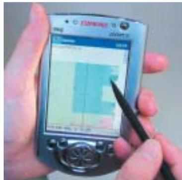
Figure 2. Dasher can be driven by eyetracker or by pointing on a touchscreen, as well as with a regular mouse.
